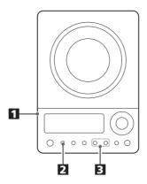
Connect the PHONES jack (audio output jack) of a portable audio player to the AUX IN jack of the CD-X10i using the supplied stereo mini plug cable.
